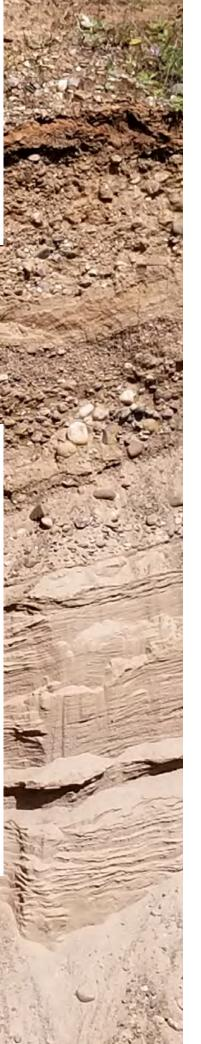
Bank height - Vertical measure from the bank toe to the top of t bank lip, irrespective of changes in the water level.
